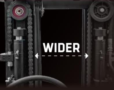
▶ The developed front lifting cylinders with smaller outer diameter give the operator superior forward visibility. The double front lifting cylinders provide better forward visibility.
