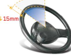
▶ The small diameter steering wheel with tilt adjustment provides the ideal operating position. The superior responsiveness of the steering wheel optimizes maneuverability even in narrow spaces.
