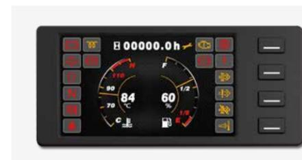
▶ Interactive instrument: The instrument adopts 4.0-inch color LCD display with four interactive buttons, and has one CAN bus communication function. The communication protocol is compatible with CANopen and SAE J1939 standards.
