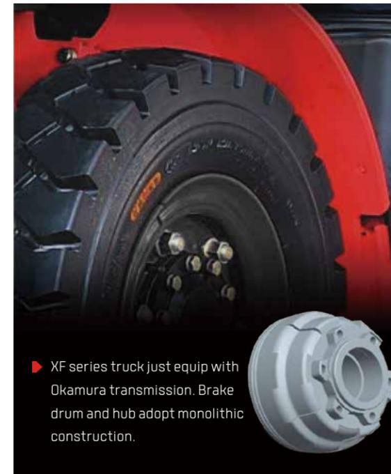
▶ XF series truck just equip with Okamura transmission. Brake drum and hub adopt monolithic construction.
