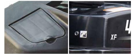
▶ The cover on the Panel can be lifted up simply to check the brake fluid.
