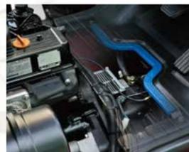
▶ In addition to rubber damper between frames and steering axle, compound engine damper and full floating power train achieve flexible connection between frames and driving system, as a result, traveling vibrations and vibrations from the driving system are significantly reduced.
